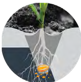
5 MICRO GRANULAR TUBE: MICRO GRANULAR PLACEMENT UNDER SEED
