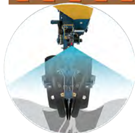
1 REAR SPRAYER ARM: HERBICIDES APPLICATION WITH A SPRAYER NOZZLE
